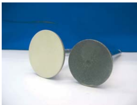
Fig. 2. The SB3.1 engine valves: with ceramic layer (on left) and with ceramic layer coated platinum
